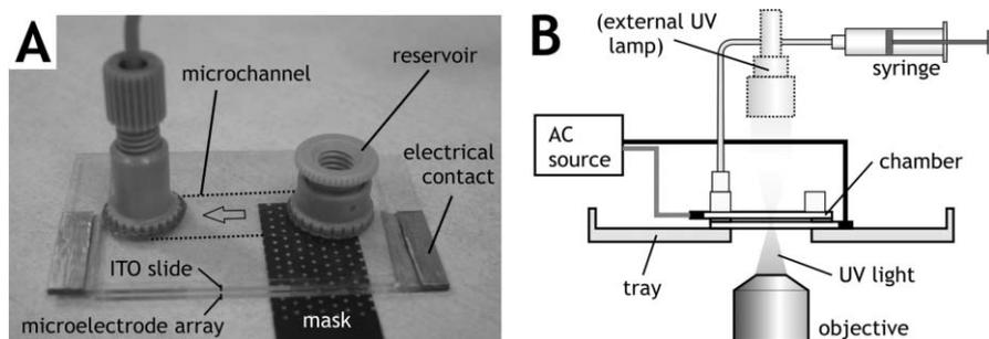
**Fig. 2** Photograph and diagram of the patterning apparatus. (A) A photomask placed beneath demonstrates transparency of the flow chamber. (B) The apparatus is loaded onto the microscope stage for visualizing cell patterning and for UV exposure by either the microscope or an external source.
