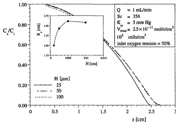
**Fig. 7** The effect of the channel height on the oxygen concentration at the chamber surface with attached hepatocytes ( $z = 0$ ). The inset shows the critical radius,  $R_c$ , where the hepatocytes are exposed to an oxygen tension,  $K_a = 5$  mmHg.
