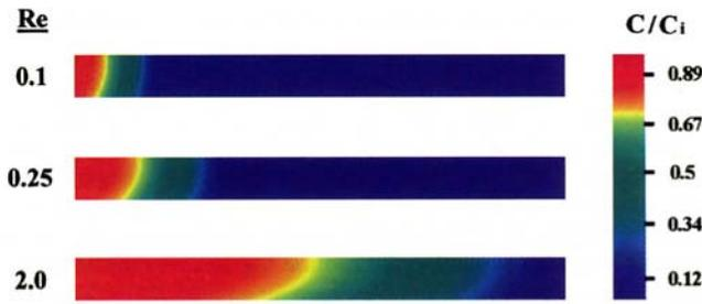
Fig. 3 The two-dimensional oxygen concentration profile in a plasma-perfused chamber. The flow conditions are  $V_{\max} = 0.4 \text{ nmol/s}/10^6 \text{ cells}$ ,  $K_m = 5 \text{ mmHg}$ ,  $H = 100 \text{ }\mu\text{m}$ , and  $10^5 \text{ cells/cm}^2$ . The Reynolds number is defined as  $Re_D = Q/\pi R \nu$ .
