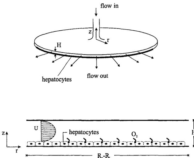
Fig. 1 Model of the BAL chambers with radial center-to-edge flow. The device scaled up in this study is composed of 10 chambers connected in parallel (piled up) with the plasma entering the chambers through the center hole ( $R_i = 0.3$  cm).
