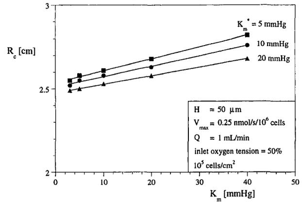
Fig. 5 The effect of  $K_m$  on the critical radius of the BAL chambers. The critical radius was calculated using three values of  $K_m^*$  (minimal allowed oxygen tension in the chambers).
