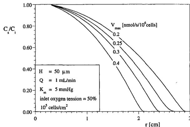
Fig. 4 The effect of the maximal oxygen uptake rate ( $V_{\max}$ ) on the dimensionless oxygen concentration at the cell-seeded surface of the BAL chambers
