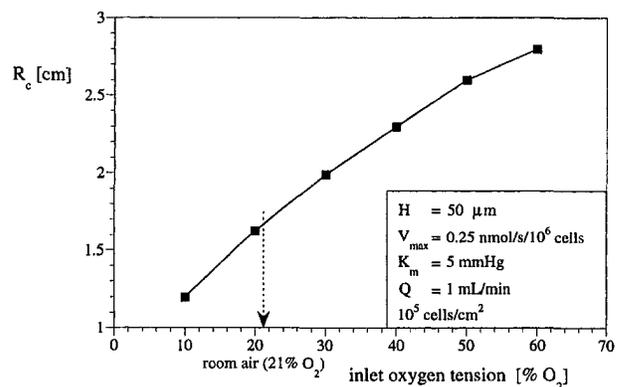
Fig. 6 The effect of the inlet oxygen tension on the critical radius. The critical radius was calculated using a minimal allowed oxygen tension,  $K_m^* = 5 \text{ mmHg}$ .
