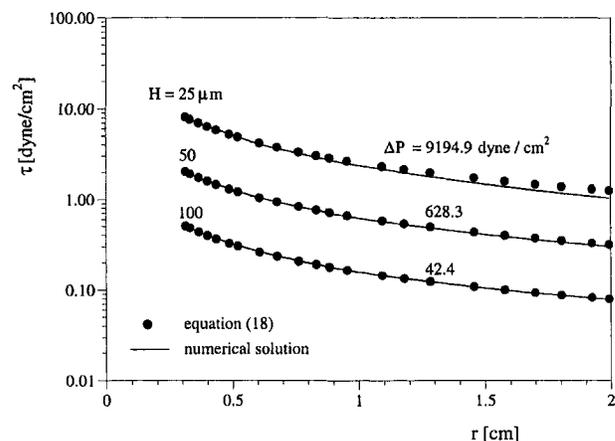
**Fig. 8** The effect of the chamber height on the shear stress and pressure drop. The total plasma flow rate is fixed,  $Q = 1$  mL/min (0.1 mL/min per chamber). The pressure drop is calculated using a chamber radius equal to 2.5 cm.
