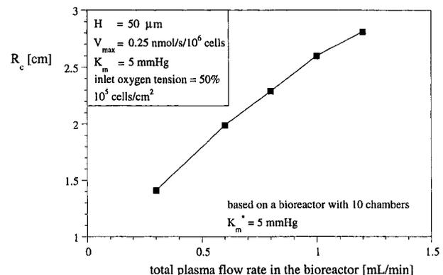
Fig. 2 The critical radius as a function of the total plasma flow rate in a bioreactor with 10 chambers. Each chamber has a plasma flow rate equal to  $0.1 \text{ mL/min}$ .
